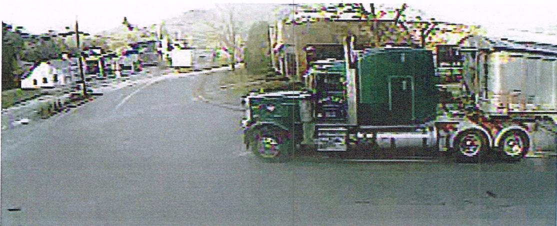
Not all large vehicles meet the design characteristics of the AASHTO WB-67; shorter trailers and vehicles with shorter wheelbases and different steering angles can maneuver through the intersection without entering the opposing lane. Of the 34 westbound trucks observed traveling through the intersection, 18 (53%) were noted to encroach into the opposing lane.
