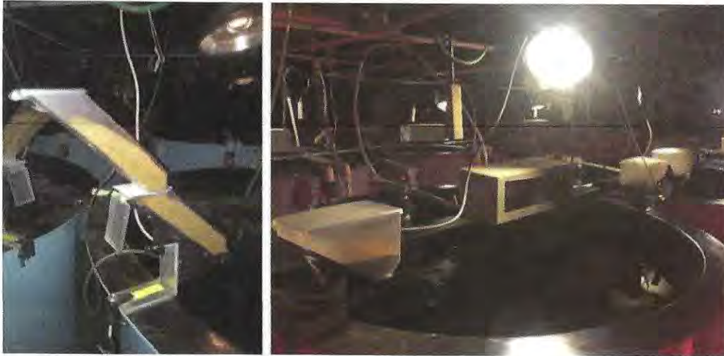
Fig. 17 Position of mounted HFS feeders on tanks: (left) a custom design modification of joining two 250-g hoppers together for increased capacity, (right) photo of 1-kg-size hoppers
