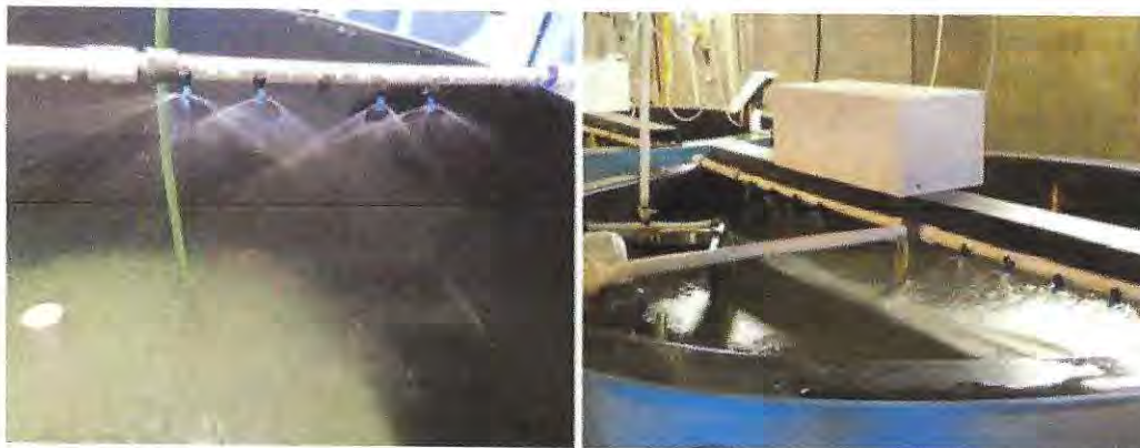
Fig. 11 Surface spray on the radial arm of the standard tank with bucket screen removed (left), spray bar spanning a self-cleaning tank (right)
