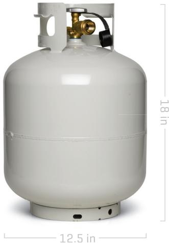
A 20-pound propane tank should be painted white or another reflective color. Tanks feature a steel footer to keep it upright, and a protective collar around the service valve. The valve will look triangular or similar to a faucet handle.
