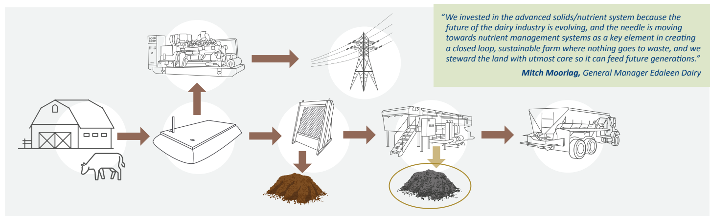
FIGURE 1. MANURE MANAGEMENT SYSTEM FLOWCHART — DVO PHOSPHORUS RECOVERY SYSTEM (SOLID PRODUCT CIRCLED).
