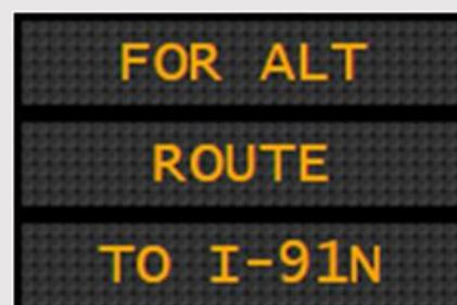
The content of Variable Message Signs that alerts travelers can change to respond to existing conditions. Messages can accommodate eight characters per line, with three lines and two phases.
