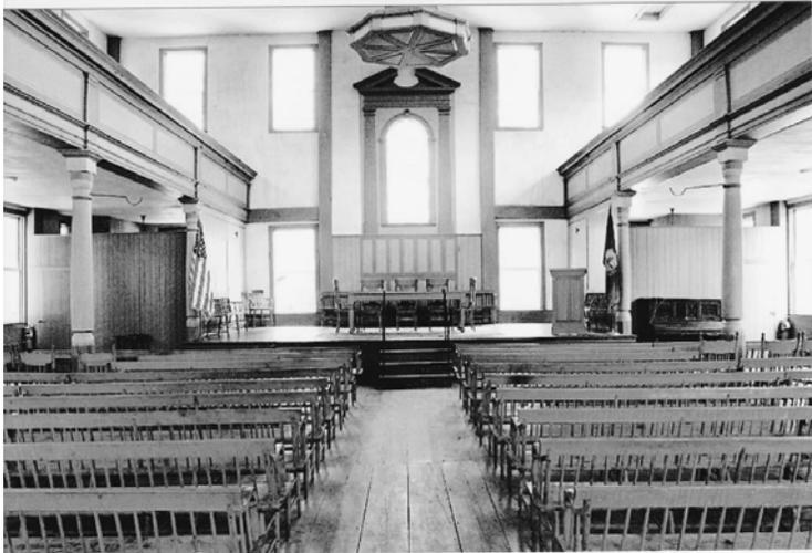
*The Town House interior after the proscenium was removed in a 1972 renovation, and the wood stoves and stove pipes taken out in 2009 for a new propane heating system.*
