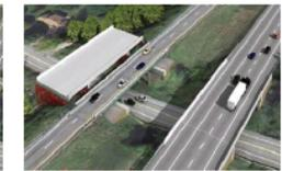
Step 3: Slide the new superstructure into place and reopen the bridge
