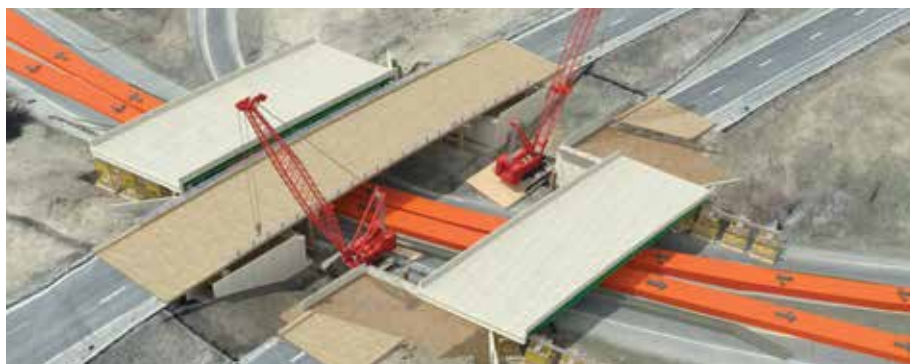
HARTFORD. Rendering of "Lateral Slide" bridge replacement project on I-91. Sliding in completed structure reduces duration of lane closures.
